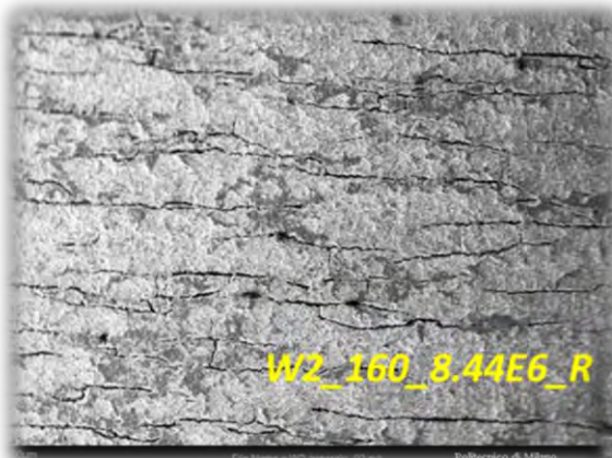
Specimen W2, \Delta S=320 MPa. Broken at 8.44 \cdot 10^6
