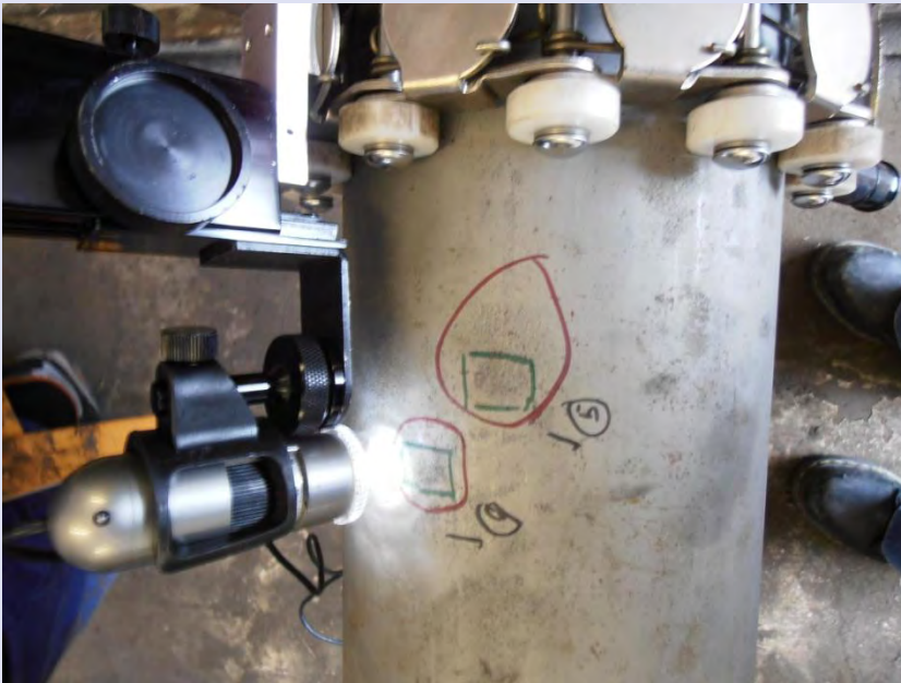
Pictures taken in Hamilton of inspected areas on axle (left) and picture of 1.5mm crack in area 9 (right)
