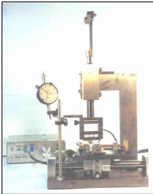
Razor blade cutting rig
