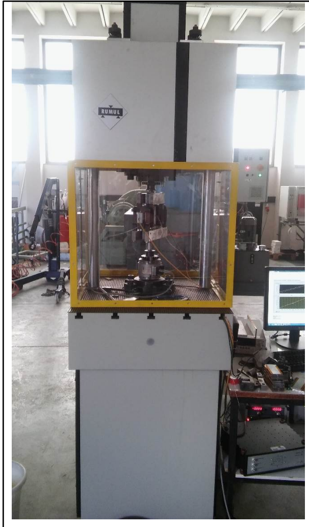
Resonant testing rig (RUMUL TESTRONIC)
