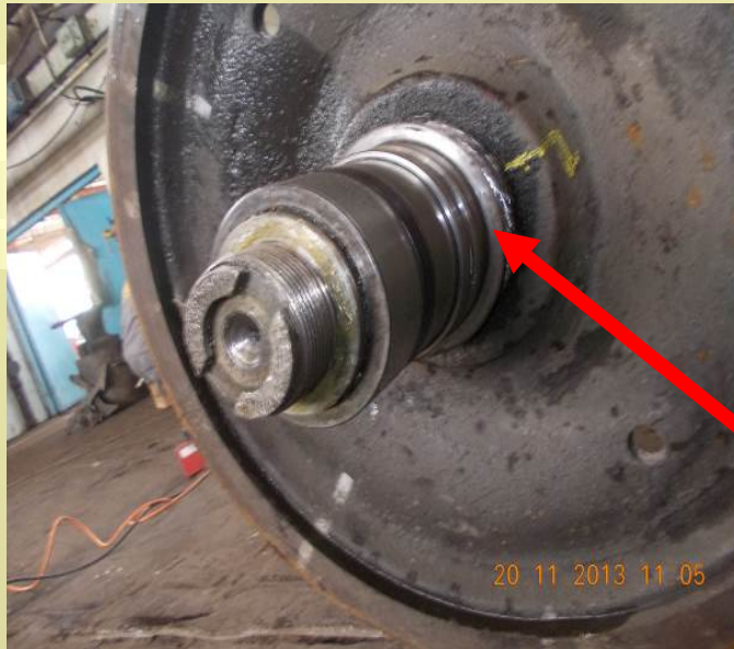
Fig. 3. Journal on the side of the railway axle where fracture has not occurred
