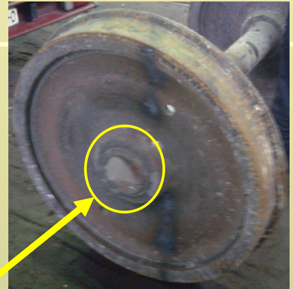
Fig. 2. The railway wheel and axle with signed fractured surface
