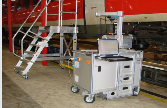
HPS-inspection device applied at a train
