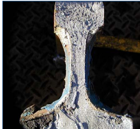
Lack of fusion
