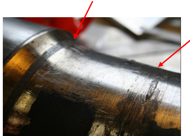
Axle with visibel traces of contact with friction
