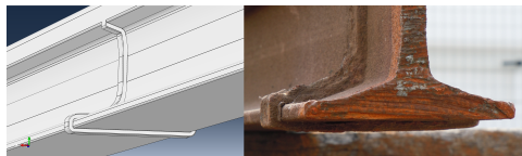
(a) comparison between model and real geometry
